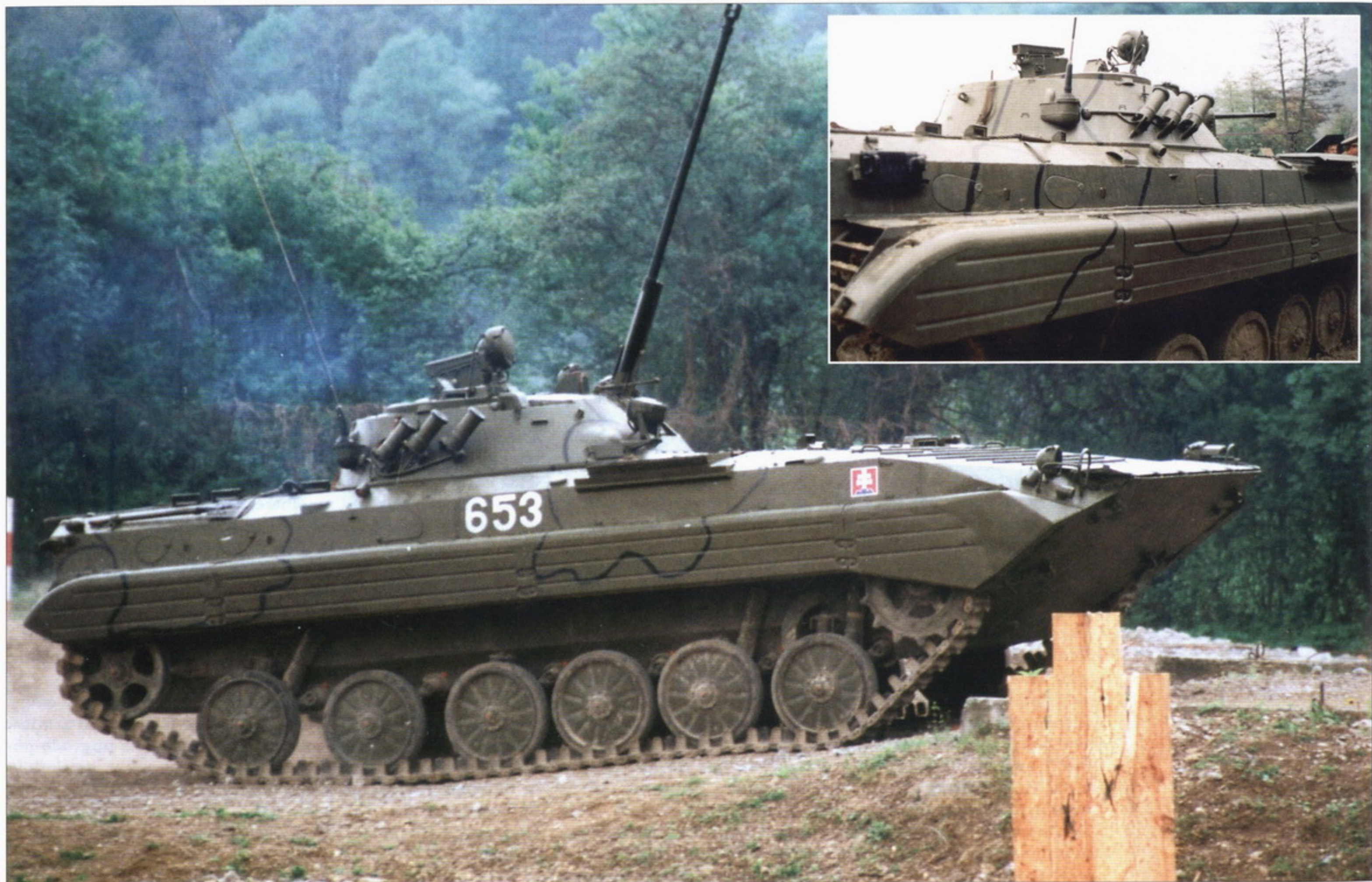
A Slovak BMP-2 with a gun at max. elevation angle – 74 degrees. Above and right: side view of the Slovak BMP-2 • Słowacki BMP-2
