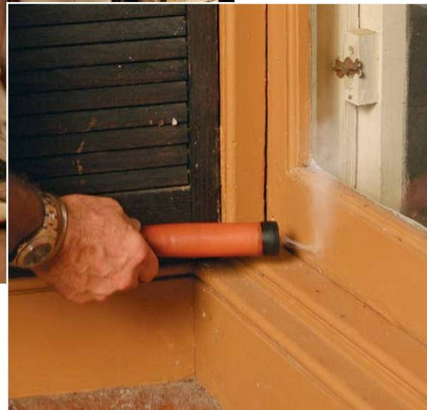
**Locating leaks.** One of the most valuable scientific tools an auditor can use is a blower door, which is mounted temporarily on an exterior-door frame. The blower door's calibrated fan pulls air through the building, measuring the amount of air leaks. While the fan is operating, an auditor uses a smoke stick to locate the leaks. Smoke pulls away from the leaky spot and toward the blower door.
